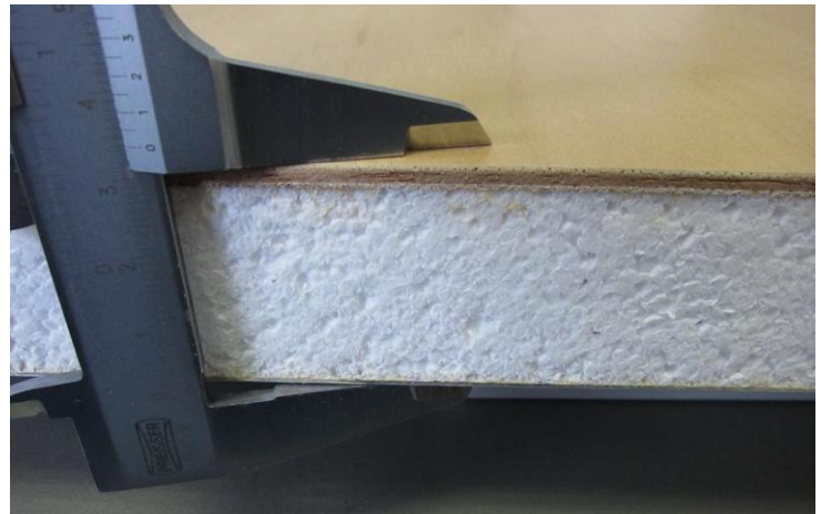
Example sandwich: aluminum - insulation - plywood
